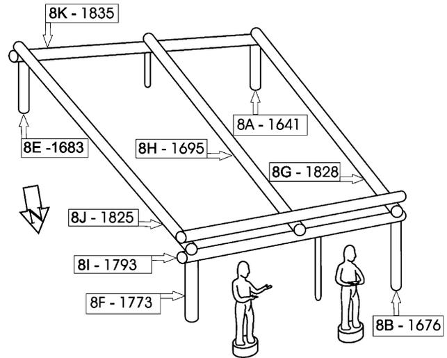
Fig. 6. Reconstructed frame of *Quaksweaqwul* showing outermost perimeter date of posts and beams established by cross-dating to living Western redcedar chronology (adapted from Mackie and Williamson, 2003).
