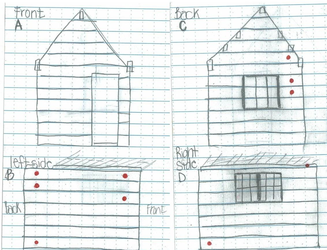
Figure 4. Field sketches of Eva Lake cabin. Red dots show approximate location of the extraction of core samples.
