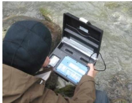
**Figure 7.** Using the HACH conductivity meter to measure temperature, conductivity and total dissolved solids.
