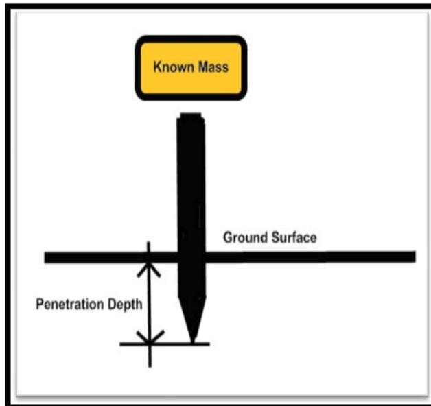
**Figure 4. Penetrometer, consists of a stick with a pointed end (199.10 g) and a weight with a known mass (926.42 g), used to estimate percent compaction.**
