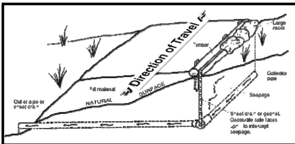
**Figure 8. Diagram showing the use of sheet drain on the uphill side of the trail to mitigate soil erosion caused by soil creep.**
