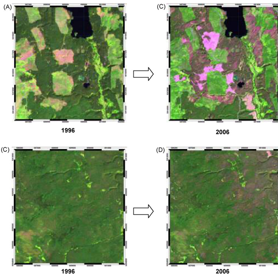
Fig. 3. Landsat TM and ETM+ image subset windows (RGB bands 543) displaying mountain pine beetle infestation (reddish-brown) and timber harvest (bright green = regenerating clearcut; magenta = recent clearcut). (a) and (b) land cover changes over a window representing a managed forest between 1996 and 2006, respectively; (c) and (d) land cover changes over a window representing an unmanaged forest between 1996 and 2006, respectively. (For interpretation of the references to color in this figure legend, the reader is referred to the web version of the article.)
