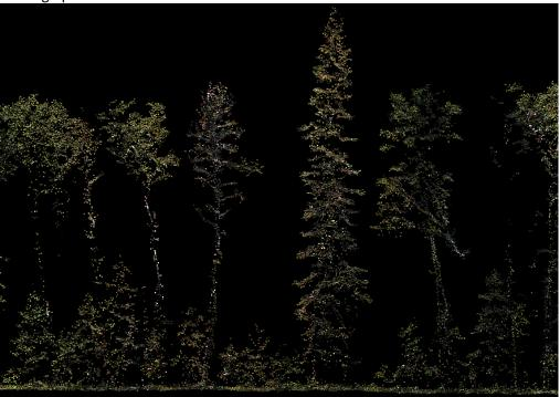
Dense, colourized lidar point cloud from University of Lethbridge Titan airborne lidar system. Image of site in NWT provided by **Maxim Okhrimenko**.
