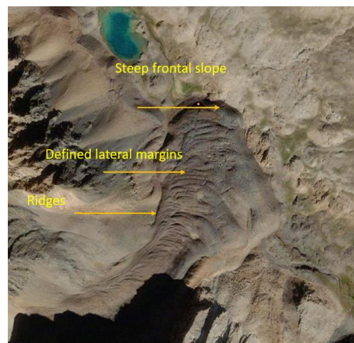
Figure 2: Active rock glacier, SA3, ESRI World imagery base layer (ArcGIS Pro, version 2.9.3) with defined, steep terminus and lateral margins. Ridge and furrow topography indicative of flow also apparent, 1:10,000.
