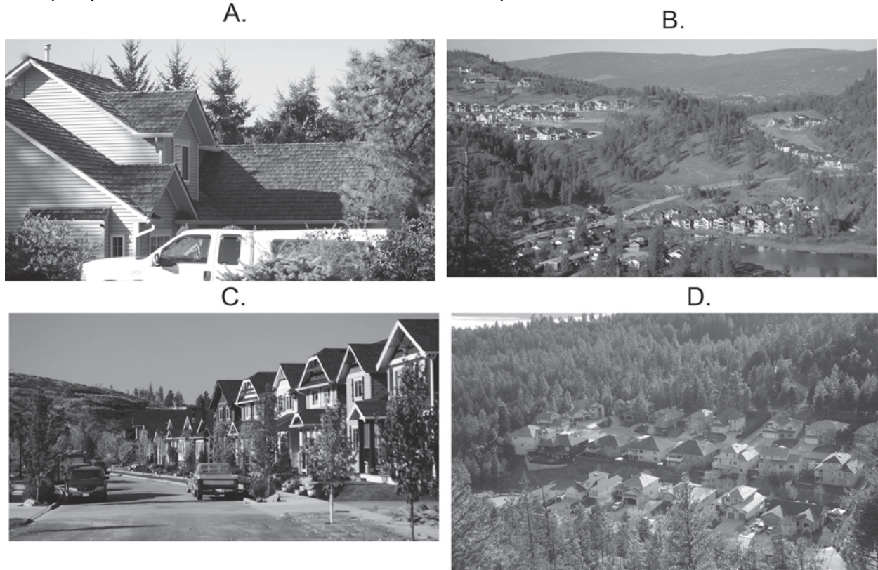
Figure 7. Existing or newly created vulnerabilities, Upper Mission and Glenmore Highlands. These include wooden roofing and siding materials (a), development in hilly intermix areas with limited egress and access (b), lack of defensible space around homes (a,d), difficulties of access for firefighting apparatus because of narrow lane with parked vehicles (c), and dense coniferous forest surrounding neighbourhoods with only one means of egress and access (d).
