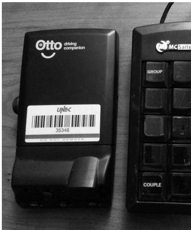
Figure 1. Persentech Otto Hitchhiker units modified to gather information on hitchhikers by pressing Group, Couple, Unknown, Female, or Male buttons. A red error button was later added.
